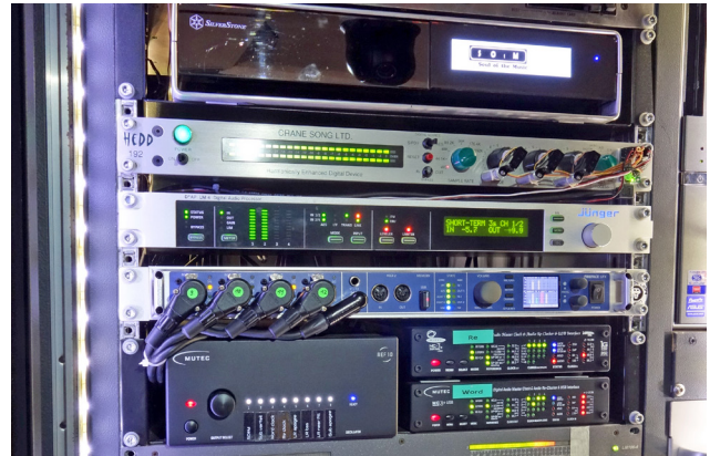
Input section of the PA system. Photo attribution: Andreas Plodek, REALHORNS SOUNDSYSTEMS
